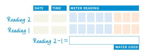
If the numbers have changed from when you read the meter the first time to when you read the meter the second time there may be a leak. If the meter has not moved, there is no leak.
