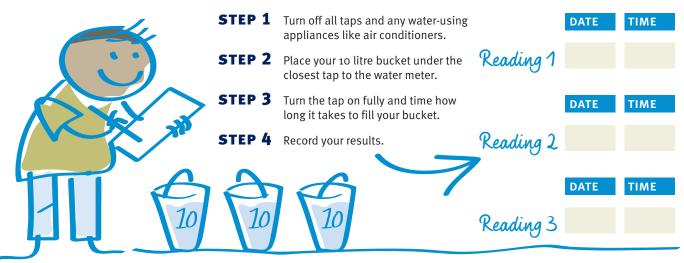
A 10-litre bucket should take less than 30 seconds to fill.
